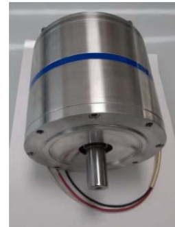
MechSTOR prototype dual-rotor ironless radial flux permanent magnet machine.
